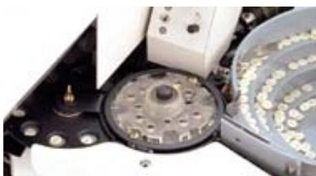
● Horizontal, forced feed mechanism
